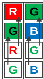
Figure 8-46 Vertical color Binning by 2
