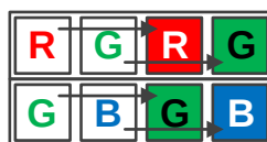
Figure 8-48 Horizontal color Binning by 2
