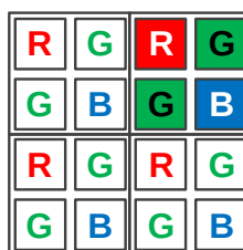
Figure 8-50 Horizontal and vertical color Binning by 2x2
