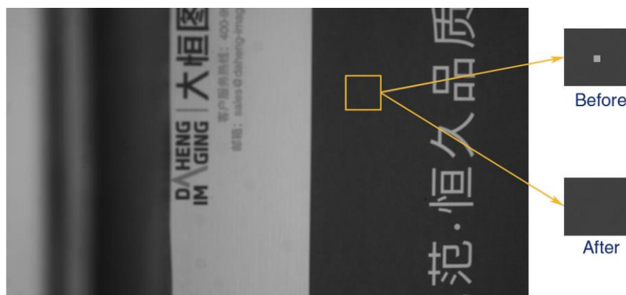
Figure 8-60 Defect pixel correction effect in actual scenario
