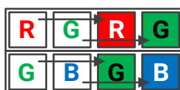
Figure 8-38 Horizontal color Binning by 2
