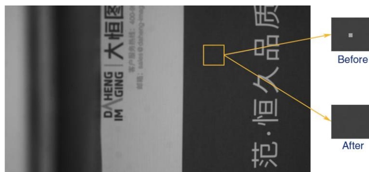
Figure 8-78 Defect pixel correction effect in actual scenario
