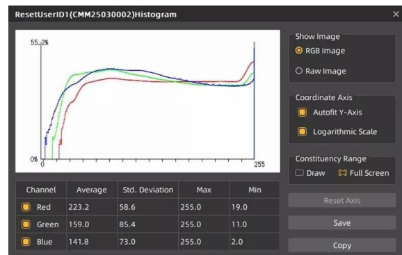
Figure 8-36 Image with 50% slope under Single Knee Point and Grey Value
