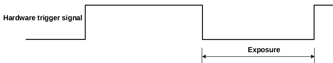
Figure 8-27 The sequence diagram in falling edge trigger of TriggerWidth exposure mode
